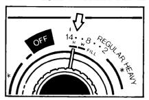
HOT WASH can be selected only in the REGULAR HEAVY Cycle. Turn the Control Knob so the pointer is on 14 or 12 minutes in the REGULAR HEAVY Cycle.
